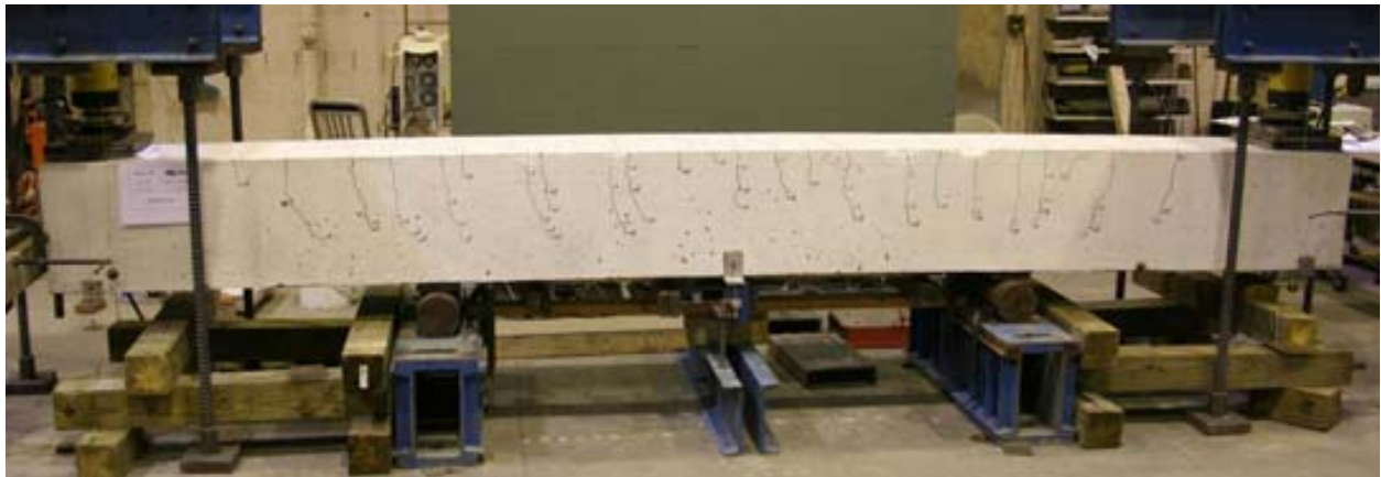
Reinforced concrete beams are being tested to evaluate lap splice lengths.
